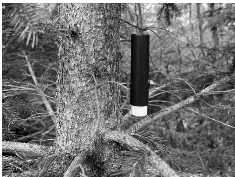
Figure 1. Example of a spot dendrometer installation on PRP 2 in the Rumburk Forest District
