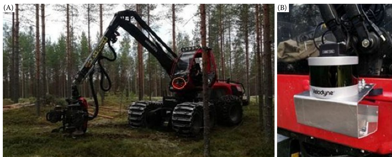
Figure 4. (A) Komatsu Forest 931.1 forest harvester (the LiDAR scanner is marked by a red circle in the front of the windshield of the cabin); (B) a close-up of the LiDAR scanner (Li et al. 2020)
