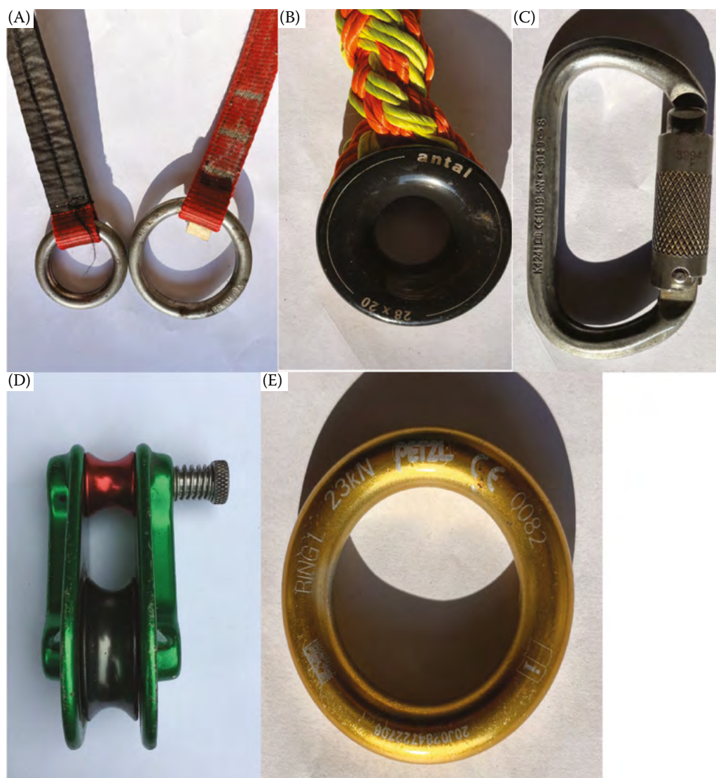
Figure 3. Tested lowering devices for the upper anchoring point: (A) Singing rock Jingle II, (B) Antal Rigging Ring L 28 mm, (C) Singing Rock Ovál, (D) ISC Silver Block, (E) Petzl Ring 48 mm
