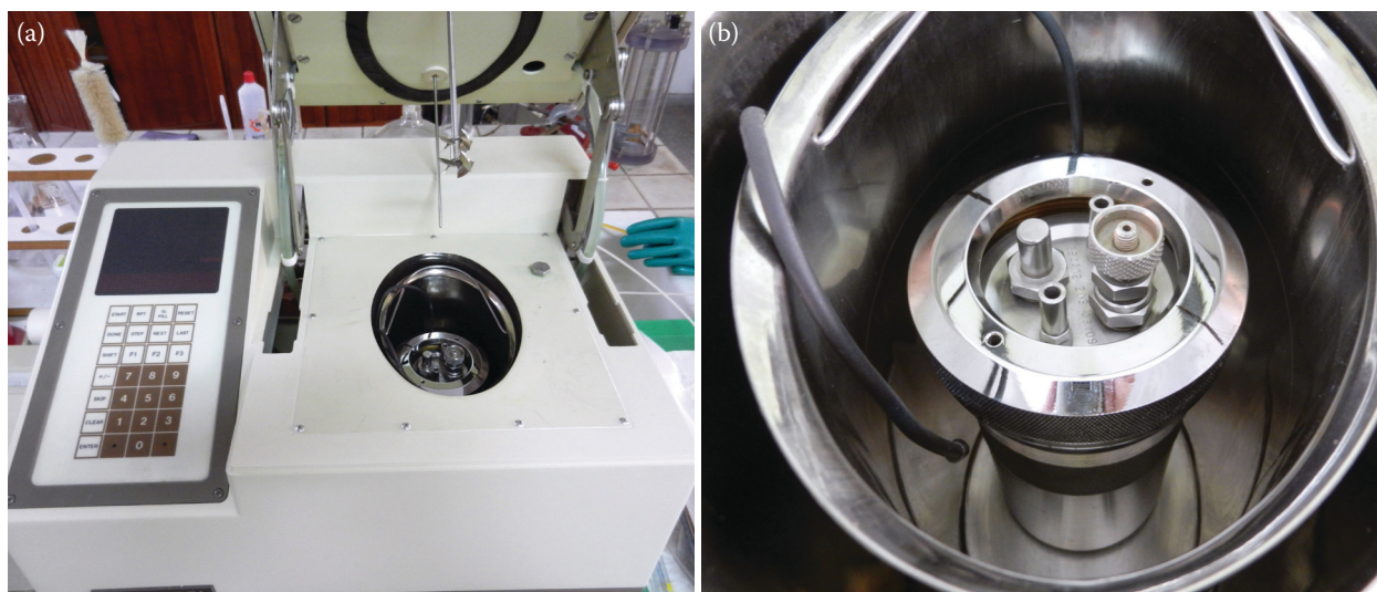
Fig. 1. Parr 1261 isoperibol bomb calorimeter (Parr Instrument Company, USA) (a), Parr 1108 oxygen combustion bomb (Parr Instrument Company, USA) (b)
