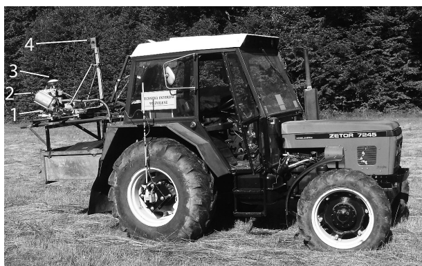
Fig. 2. RIEGL VMX-250 mobile mapping system – MMS (RIEGL Laser Measurement Systems GmbH, Austria) mounted on a Zetor Horal 7245 tractor (Zetor Tractors, a.s., Czech Republic). Two digital cameras (1) and VQ-250 mobile laser scanners (2) are placed on the side of the MMS measuring head, GPS antenna (3) is placed on the top and panoramic camera (4) above the MMS measuring head
