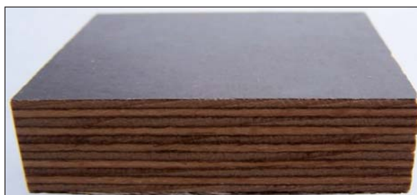
Fig. 1. Variant 1 – plywood with fibreglass (11-ply, thickness 16 mm)
