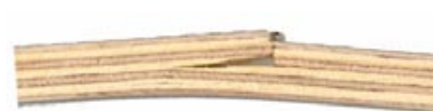
Fig. 28. Rupture of fibres in the tensile zone of the specimen in a combined plywood 15 mm thick
