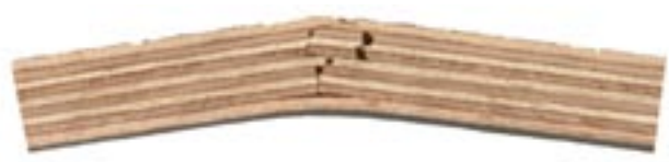
Fig. 27. Fibrous fracture along the height of the specimen in a beech plywood 15 mm thick
