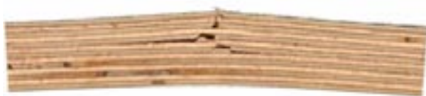
Fig. 29. Rupture of fibres in the tensile zone of the specimen in a beech plywood 18 mm thick
