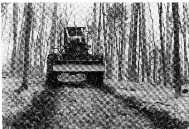
4. Eliminace prokluzu hnacích kol stroje omezuje škody na pojezdové dráze. — If the slip of the driven wheels is eliminated, the damage of the track is reduced
